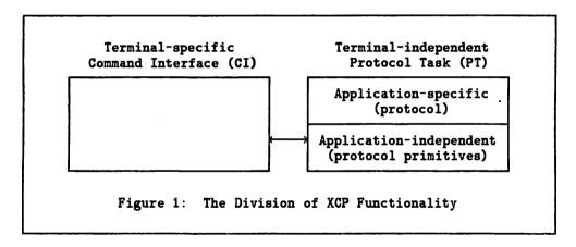
The CI interacts directly with a person at a terminal, and can be thought of as the user's front end. It formats the screen, performs command recognition, prints messages on the screen, and interacts with the PT through the exchange of messages. These messages represent either user-instigated commands or choices made in response to "demands" from the PT as it executes the protocol. There is one CI per active user.
